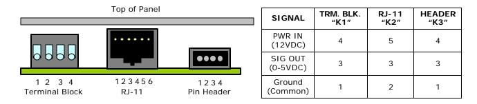
Figure 3.4 – Sensor Connector Signals – Sensor Head Side
