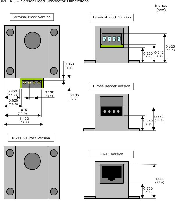
FIGURE. 4.3 – Sensor Head Connector Dimensions
