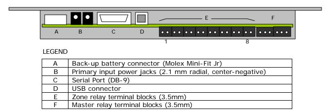
Figure 3.2 – Location of Panel Sensor Connectors
