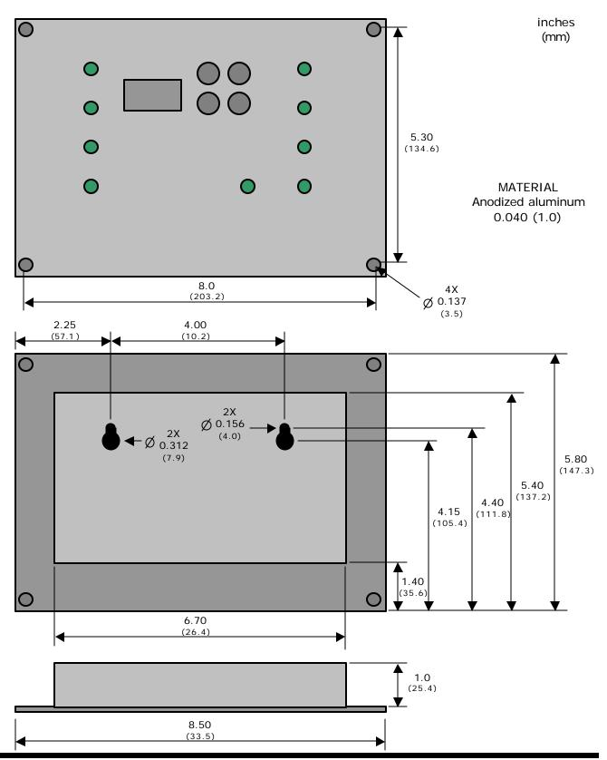
FIGURE. 4.2 – Sensor Head Dimensions
